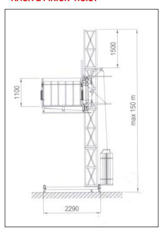
A single mast dual purpose hoist designed to carry 2000kg SWL or, with the addition of an overhead protection piece, can accommodate 7 passengers in transport platform mode.
